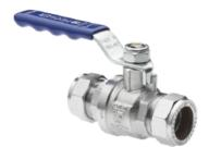
**Isolating valves** are designed to stop a fluid in a pipeline to allow maintenance or repair of a section of tube or piece equipment downstream of the valve.
