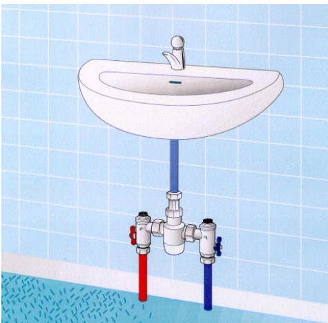
Single tap with pre-set mixed temperature from exposed under-basin TMV
