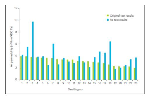
Figure 9. Air leakage retest results for 23 homes tighter than 10  $m^3/(h m^2)$ -NHBC (2011)
