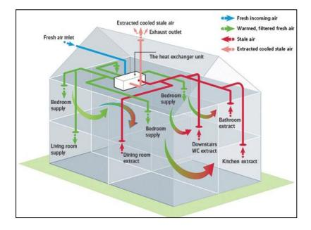
Figure 12. Mechanical ventilation with heat recovery system (MVHR)
