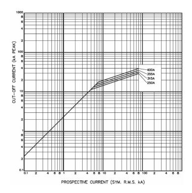
FIG. 2B 250-400A BS 88-2 FUSE TYPICAL CORRESPONDING CUT-OFF CURVES
