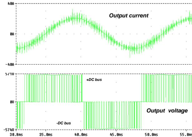
**Figure 6 – Typical PWM voltage and current motor waveforms**
