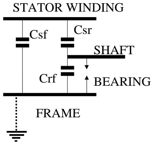
**Figure 11 - Capacitive discharge current equivalent circuit**
