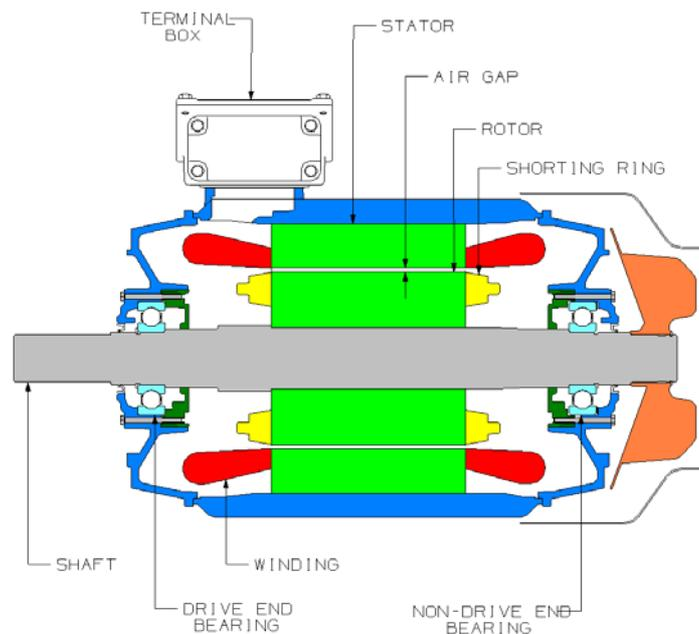
**Figure 1 - Longitudinal view of an a.c. induction motor.**
