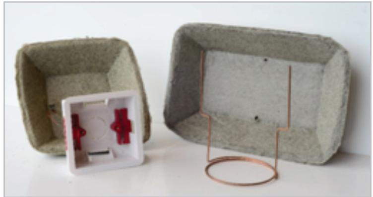
Intumescent pads are applied as adhesive pads to the inside surfaces of the mounting box:
