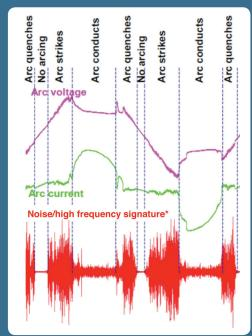
This diagram illustrates a typical arc fault signature. The noise / high frequency signature exceeds 50 Hz and can be kHz or MHz thus allowing the detection of an electric arc fault by an AFDD.
