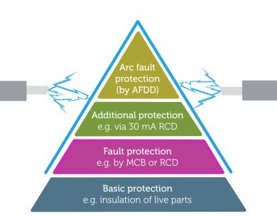
AFDDs provide additional protection that is not offered by MCBs and RCDs. AFDDs detect low level hazardous arcing that MCBs, Fuses & RCDs are not able to detect.
