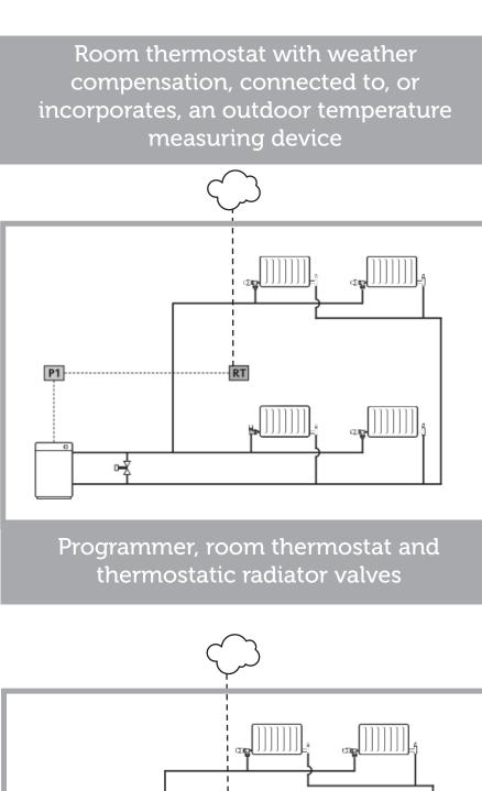
Image: constant and thermostatic radiator valves
