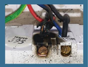
The following illustrates the development of an arcing fault as a result of conductor damage.
