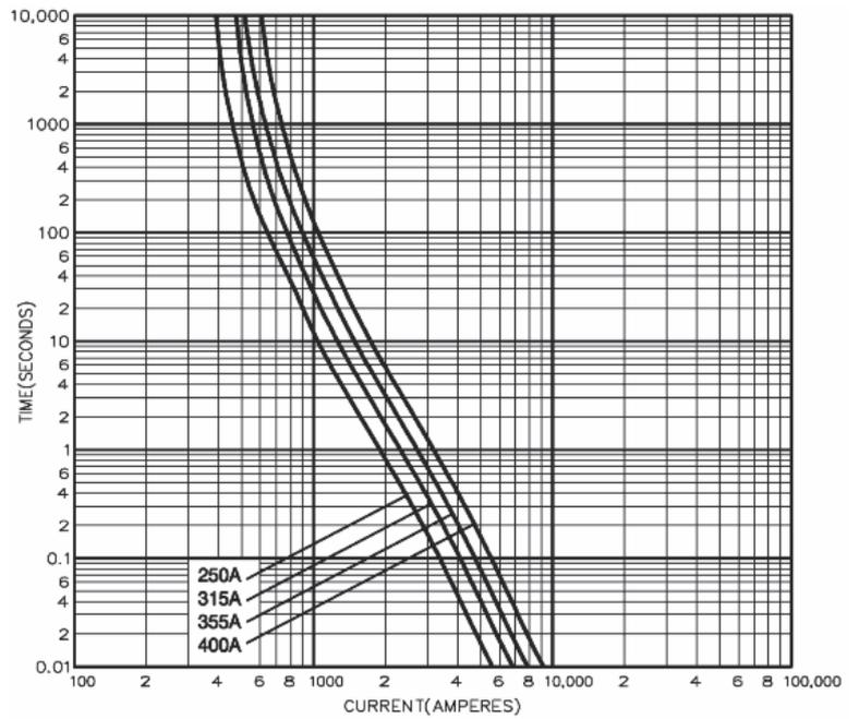
FIG. 2A 250-400A BS 88-2 FUSE TYPICAL TIME/CURRENT CHARACTERISTICS
