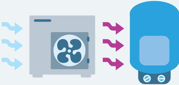
Using heat pump technology as mentioned above, a hybrid solution is either an integrated heat pump with boiler in a single box, or a separate heat pump and boiler operating bivalently i.e. simultaneously. Typically, the heat pump will supply the heat whilst supplementing the production of higher temperature hot water with the boiler.
