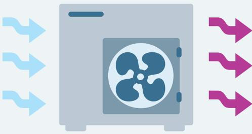
Heat pumps use a reverse refrigeration cycle to generate heat, drawing in low temperature ambient heat from the ground, air or water and turning it into high temperature heat. A heat pump's efficiency is expressed as a seasonal performance factor (SPF). If an SPF of 3 is claimed, this means a single unit of electricity used by the heat pump can generate 3 units of heat. This high efficiency is important when considering the reduced peak power demand required to deliver peak heat demand.
