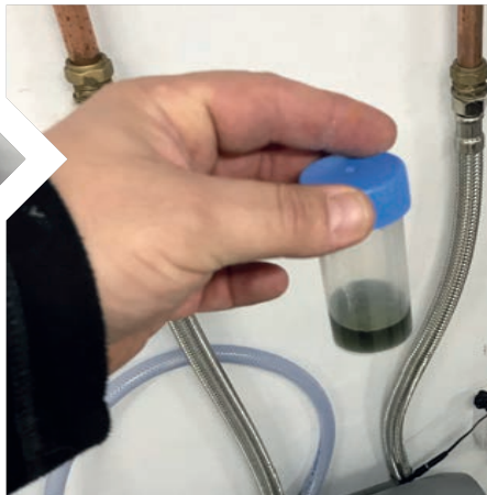
05 Use a hard water test kit to ensure you identify the correct water hardness level for your customer's softener
