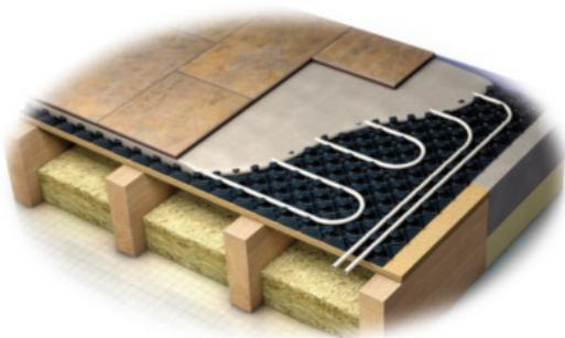
**Low section grid/levelling compound systems:** A profiled plastic panel designed to house the underfloor heating pipework and levelling. Some boards are available with an adhesive backing to help installation. The finished depth tends to be between 15 and 22mm.
