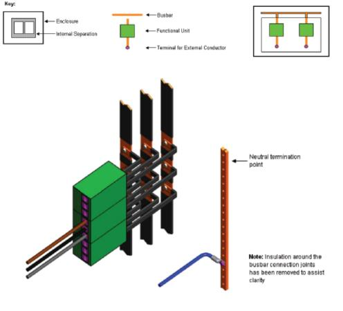
The above illustration uses the "Integral Housing of the Device" as a means of separation.
