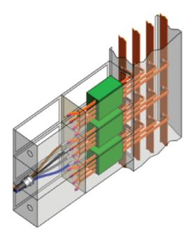
The above illustration uses "Partitions and Barriers" as a means of separation.
