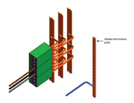
The illustration above is Form 3a where the Integral Housing of the device is the means of separation and the arrangement is regarded as 'Group Mounted'.
