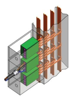
The above illustration uses "Partitions and Barriers" as a means of separation. Cable terminations are integral to the device.
