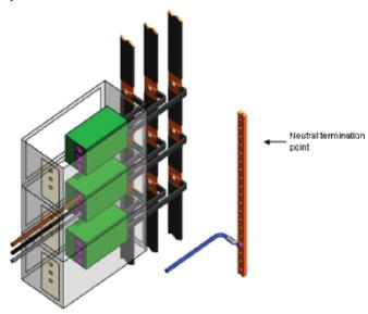
The above illustration uses "Partitions and Barriers" as a means of separation and is referred to as **Compartmentalised.**
