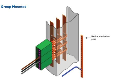
The above illustration uses the "Integral Housing of the Device" as a means of separation and is referred to as **Group Mounted**.
