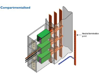
The above illustration uses "Partitions and Barriers" as a means of separation and is referred to as **Compartmentalised.**
