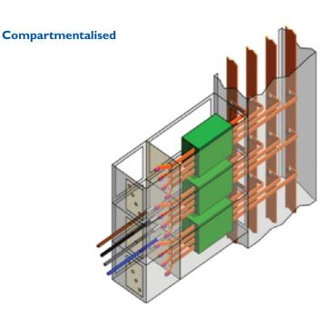
The above illustration uses "Partitions and Barriers" as a means of separation and is referred to as **Compartmentalised.**
