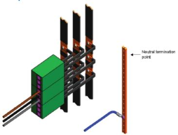
The above illustration uses the "Integral Housing of the Device" as a means of separation and is referred to as **Group Mounted**.
