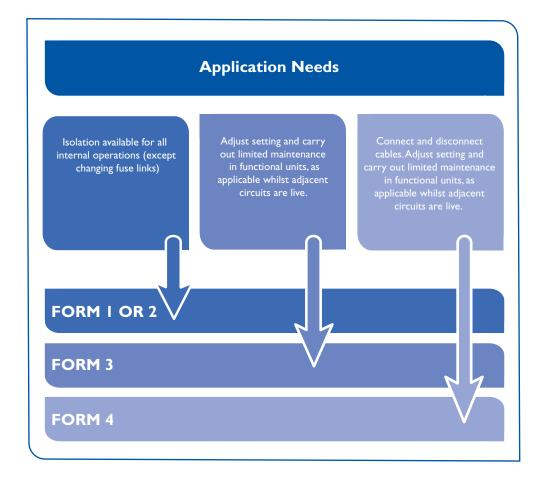
Having established the fundamental form for separation needed for an application, specific details must be considered. The IEC and EN versions of 61439-2 divide Forms 2, 3 and 4 into two sub categories. However, within the requirements defined in the standards there are three fundamental ways of providing separation:
