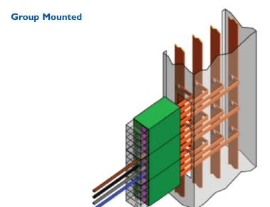
The above illustration uses the "Integral Housing of the Device" as a means of separation and is referred to as **Group Mounted**.
