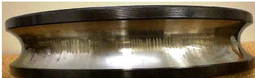
**Figure 18 – ‘Characteristic ‘fluting’ wear of inner race**
