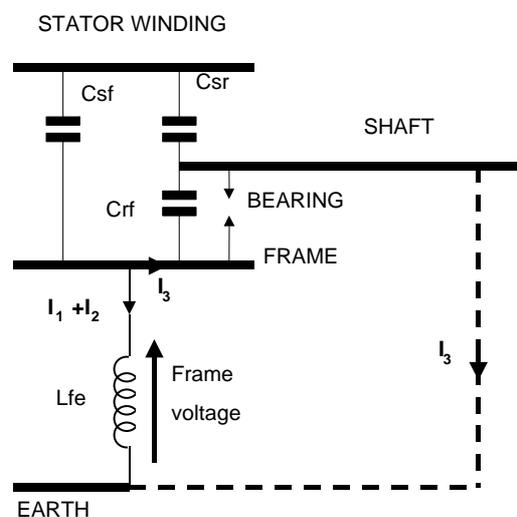
**Figure 14 - Shaft grounding current equivalent circuit**
