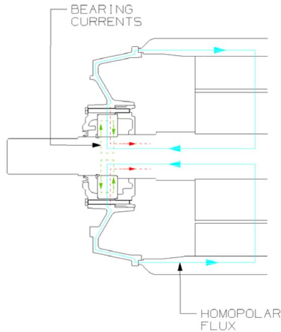
**Figure 3 - Homopolar fluxes around stator, rotor and shaft**
