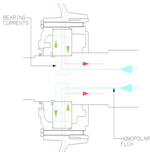
**Figure 4 - Currents adding in a bearing**
