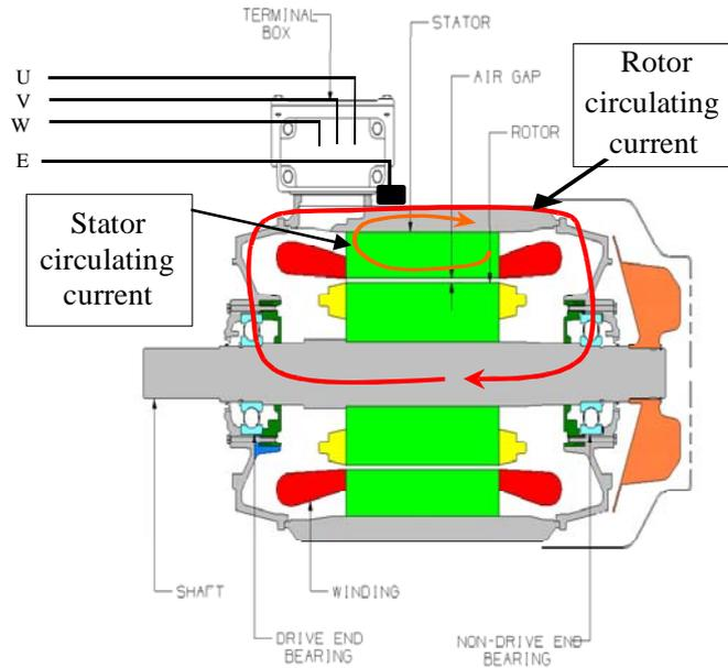
**Figure 16 - Induction of rotor circulating current**
