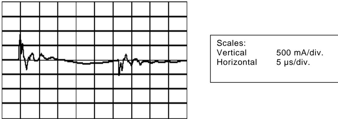
**Figure 10 - Typical waveform of motor frame earth current**
