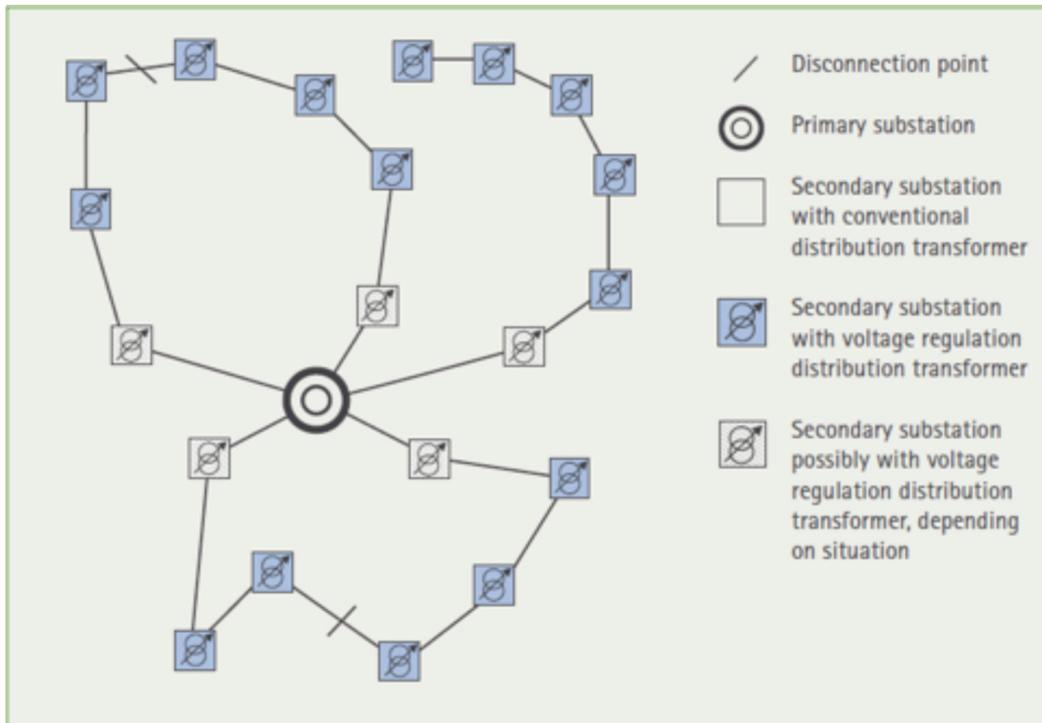
Figure 3: Use of voltage regulation distribution transformers in all parts of the grid with a focus on the medium-voltage grid
