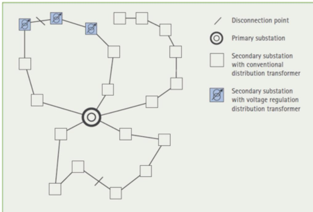
**Figure 2: Feeder-based use of voltage regulation distribution transformers with a focus on the medium-voltage grid**
