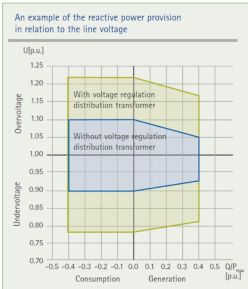
Figure 6: An example of the reactive power provision in relation to the line voltage
