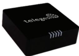
**2. Gateway CAD:** This provides a bridge between the data generated by the communications hub (gas and electricity consumption) and WiFi, ethernet port, 3G or 4G cellular, mesh radio or another alternate WAN technology. It can transmit data either inside the property or to an external internet location.
