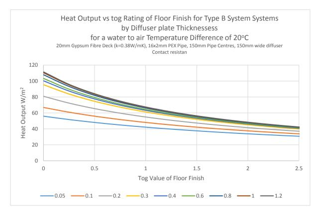
It can be seen that the thinnest aluminium diffuser plate of 0.05mm (typically a foil based product) will have a heat output of around 40W/m² when used with a typical 1 tog floor covering. Increasing the thickness of the foil to 0.6mm increases the heat output by 62.5% to 64 W/ m². A further increase to 1.2mm results in a heat output of 67W/ m².
