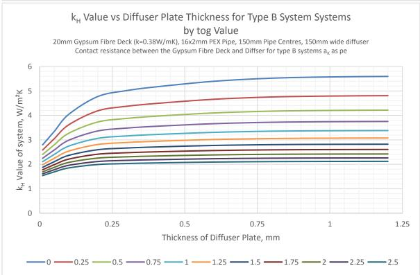
Whilst the above graphs are interesting let's put this data into a typical UFH heating system where we have an average heating water temperature of 40°C and an air temperature of 20°C, giving a temperature difference of 20°C.
