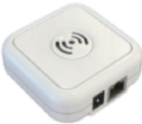
The Consumer Access Device (CAD<sup>2</sup>) provides the link between the Smart Grid and the rest of the consumer's world, opening the door to the future of the Smart Home. It speaks one messaging protocol to the metering network within the home, whilst potentially speaking multiple protocols to individual consumer devices and external services.
